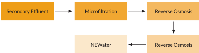
Figure 8.2: Treatment Process Flow Diagram of the NEWater Reclamation Plant, Singapore
